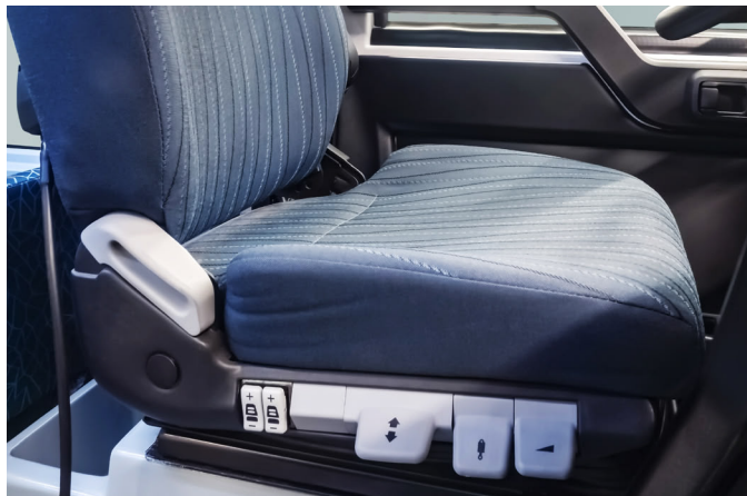
Adjustable Pneumatic Driver Seat With Arm Rest
